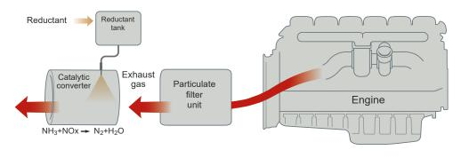
The emissions of particulate matter are filtered through a ceramic structure, that only allows particles smaller than a defined size to pass. When the filter is filled with soot particles to a specific amount, it is regenerated automatically.
